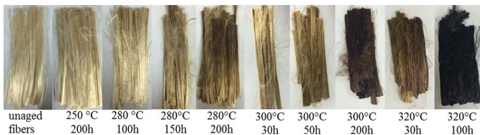
Figure 4. Photographs of co -PSA fibers thermal-oxidative aging at different conditions. [Color figure can be viewed in the online issue, which is available at wileyonlinelibrary.com .]
